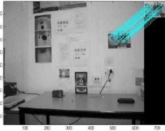
Figure 6-A sample of matched keypoints provided by the SIFT operator
